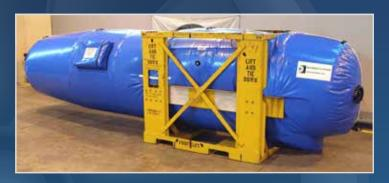
The preservation system is monitored by observing an Environmental digital indicator which is located on the side of the WVR Aero-bag and is capable of reading relative humidity, temperature and due point inside the Aero-bag.
