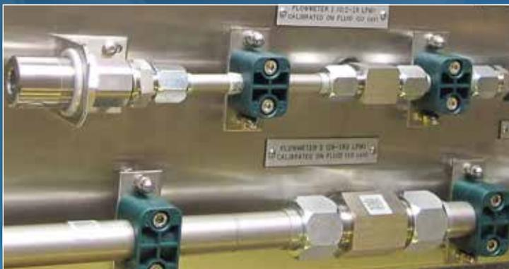
A small flow control needle valve is mounted in line with the low flow flowmeter.
